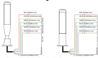
Remark: Connect the wire according to the colors if necessary.
