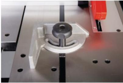
Infinitely adjustable angle stop from  $-45^\circ$  to  $45^\circ$
